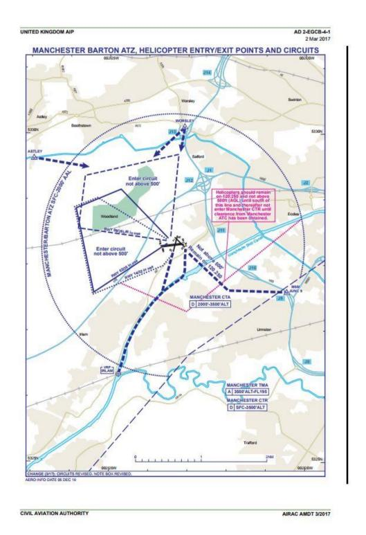
4.1.2 **Astley:** Pilots should enter the helicopter circuit (not above 500 ft agl) and then position to the Airfield, landing at either the Runways 20, 14 thresholds or directly into Helicopter Training Area North (HTAN).
